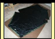
Here's the liner with shockcord housings and corner attachment loops all sewn on. Next, we're going to sew the darts together.
