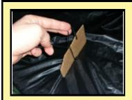
Make a mandrel out of cardboard. For two layers of insulation, mark it off to 2". That's the max height of the insulation. I don't think it ever gets that high, but that takes into account the nylon and a little room for error. Put the needle in on the liner so that the knot will be on that side. For each loop, tie it around the mandrel to get the size right. I triple knot each one very tightly and trim the ends to about a half inch.
